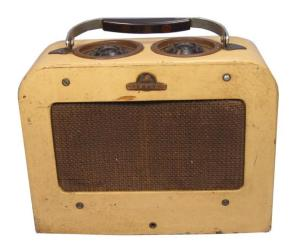
The ply wood casing is of low sophistication requiring only a small amount of steam bending to round the shoulders.
