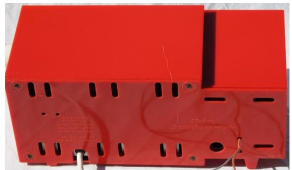
Indifferent ventilation leads to cracks in the main case.
