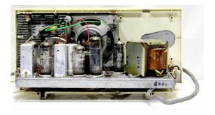
The local oscillator circuit feeding into the 6AN7 is an Armstrong configuration using a coil tuned by one gang of the tuning capacitor coupled to a "tickler" coil providing positive feedback for oscillation.
