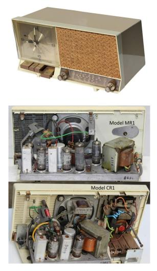
The clock radio has a smaller chassis facilitated by using a 6DX8 triode-pentode to reduce the valve count to four.
