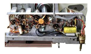
A look under the chassis shows a tangle of components wired point to point. Circuit boards were quickly taken up for transistor radios, but old ways of construction and wiring died hard for valve radios. A relatively small tuning capacitor is among the few "modern" components.
