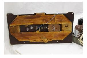
The antenna coil was open circuit and the single break was easily located and repaired. Provision is made for adding an external aerial and this would be essential in most locations, given that this radio has no RF amplifier stage.
