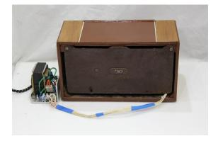
The original case is most easily described by the word *wonky*. Some replacement bits and generous PVA gluing restored physical integrity. There was little scope for anything but a complete sanding-back of the case surface. Accented sections were painted with near original colours. The whole case then had several coats of gloss polyurethane sprayed on.
