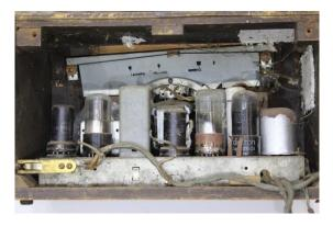
A gold 6.5mm mono audio socket can be seen at rear left mounted into the wooden case. This accepted output from a turntable to play records and switched the radio-feed out of circuit when a plug was inserted. The same stock of heavy braided shielded wire used for the pick-up connection was also used to connect 6V DC to the vibrator and return high tension from the vibrator. Those vibrator connections were made using an Australian general purpose 240V power plug and socket.
