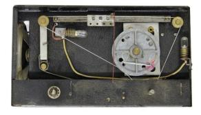
A diffuser card for the dial is retained by ties anchored in grommet holes.
