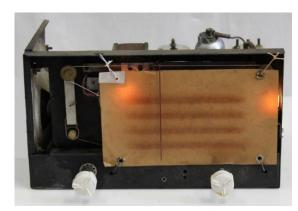
Restoration included replacing the 0.02 uF audio coupling capacitor to the 6V6 and the 6V6 0.003 uF plate decoupling capacitor. A new three core power cable was installed. With these minor changes the radio worked well, with everything performing to specification.
