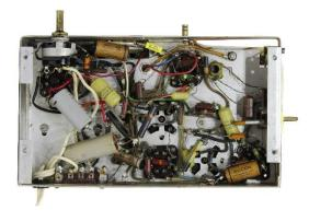
The underside of the chassis is well set out for easy replacements. Some critical capacitors had already been replaced so only the plate bypass capacitor to the 6V6 was additionally replaced. The radio performs well within the limitations of four valves and a five inch Rola speaker.
