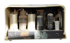
As seen from the rear, the top right hand corner of the case was chipped off. The gap was filled with two-part car-body filler, profiled to shape, then painted ivory to match the case.
