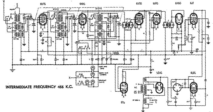
band. It was possible that the 6. 3V line, which is capable of high current, was causing the sparking and burning. This was the easiest cause to investigate so the 5Z4 rectifier was removed to eliminate high tension circuits. It was soon evident that the 6. 3V was not the source of the arcing. There were three more switch sections on the wafer.
