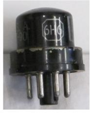
831 is a top shelf design with nine separate valve envelopes. Unusually the diodes for AGC and detection are in a stand alone 6H6 miniature octal valve. This small valve is nevertheless enclosed in a full size valve shield.
