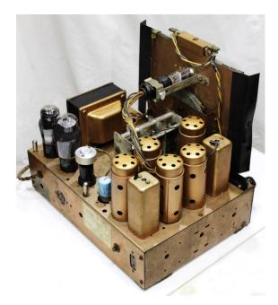
And so it proved to be. First power up was without the high tension rectifier. This tests the power transformer for stable operation and lights up the dial lamps (all came on). When the valves and speaker were added the radio worked. This was good news, but the distortion and crackle were not so welcome. Power consumption at this time was 72W; high but not too surprising. The first fault to tackle was the distortion. My immediate suspect was low bias to the 6L6 output pentode.
