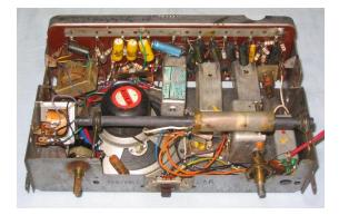
Printed circuit boards were known at the time, but none of the radios shown here used one. In my collection Admiral is the only Australian manufacturer from the 1950s to use printed circuit boards in both their valve and transistor radios. See further comment on the early use of printed circuit boards in Silicon Chip *Vintage Radio* May 2019, "The admiral 5ACW valve radio".
