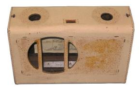
This transistor radio and the contemporary Stromberg Carlson valve mantel radio (the Baby Grand) share the same model Rola 5F speaker for output. Both cases provide comparable baffling to the speaker.
