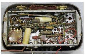
This design has one enormous advantage. After removing the four screws securing the chassis at the base, the whole radio (knobs and all) separates cleanly from the case. Some other manufacturers (notably STC) also featured partly recessed knobs at the time.
