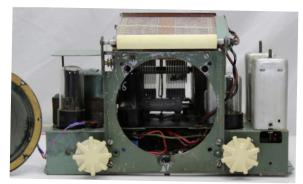
The 6.3V lines to the dial globes had badly perished rubber insulation and were replaced. A number of rubber wires under the chassis were likewise perished, but many were impractical to replace due to bad layout of components stacked on each other. During restoration care was taken to minimise disturbance of any reasonably intact rubber insulated wires, because beads of rubber can fall off exposing bare wire. In the end the radio came back to life without any sparks.
