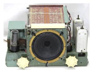
The unusual chassis layout had a downside. The 6V6 and HT ballast resistor are under the dial and only easily accessible when the speaker is removed.
