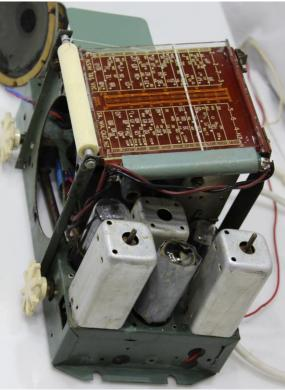
With the radio electrically functional all that remained was to restring the tuning drive. The refurbished case was added and the restoration was complete. The rear view is not the radio's best angle, but it makes a fitting end to the narrative.
