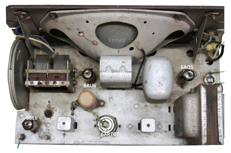
The photo of the top of the chassis shows slightly grubby metalwork and discoloured vanes in the tuning capacitor. Initially I was keener to see if the radio worked than to spruce up the appearance. This turned out to be an unfortunate choice of priority.
